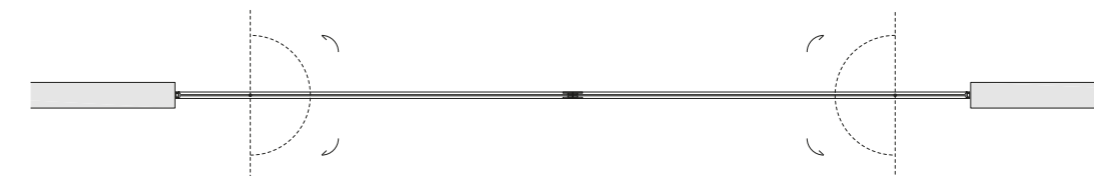
Pivot Flipping laterale 2 ante - Lateral Flipping Pivot 2 leaves doors
