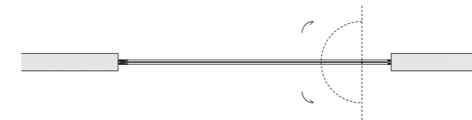
Pivot Flipping laterale 1 anta - Lateral Flipping Pivot 1 leaf door
